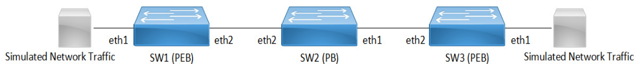
Figure 2-3: Single provider bridge configuration
