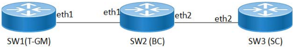
SMPTE PTP Configuration Topology
