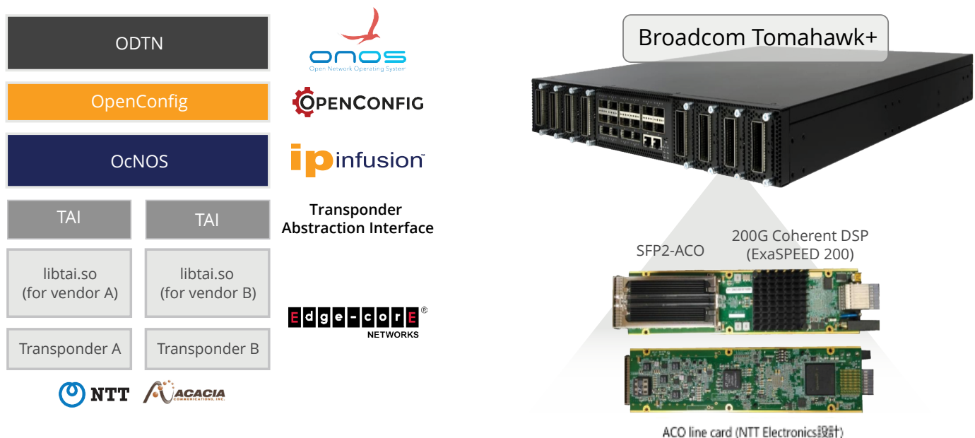
Figure 6: Fully integrated Packet Optical Transponder.
