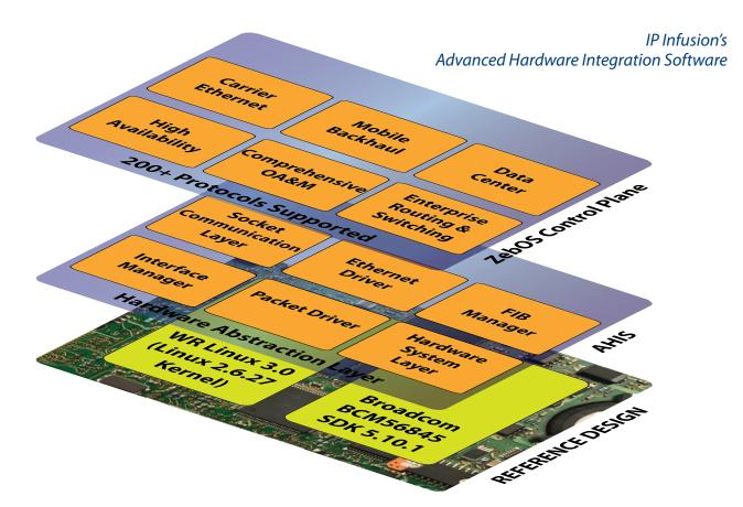
IP Infusion's AHIS integrates the control plane with the reference designs of the popular chipsets in the networking industry. The software integration is built using a vendor-specific chipset SDK and reference operating system recommended by the vendor. The integrated software solution enables you to accelerate the delivery of next generation networking solutions.
